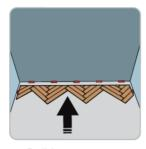
13. Build up some more rows this will help to strengthen the floor, use the same method as before, begin the row from left to right finish with a cut as previously used then work back right to left.
