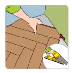
16. To give additional strength to the final boards run some suitable flooring adhesive into the groove to help secure the smaller planks.
