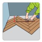
10a. Using a tape mark off positions to form a cut line across the run of flooring maintaining an equal distance to the starting wall.
