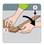
2. To connect plank No.2 (Type B) press the long side of the plank at an angle into the short side of the previous installed plank, folding the second panel to the floor will lock them together, checking that the grooves form a continues line
