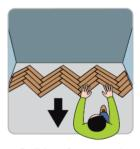
9.Build up four complete rows using the same method to give a body of flooring ready to be cut or scribed to the starting wall.
