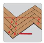
11. The floor will need to be taken apart and cut, numbering the planks will allow them to be kept in order. Cut along the marked line
